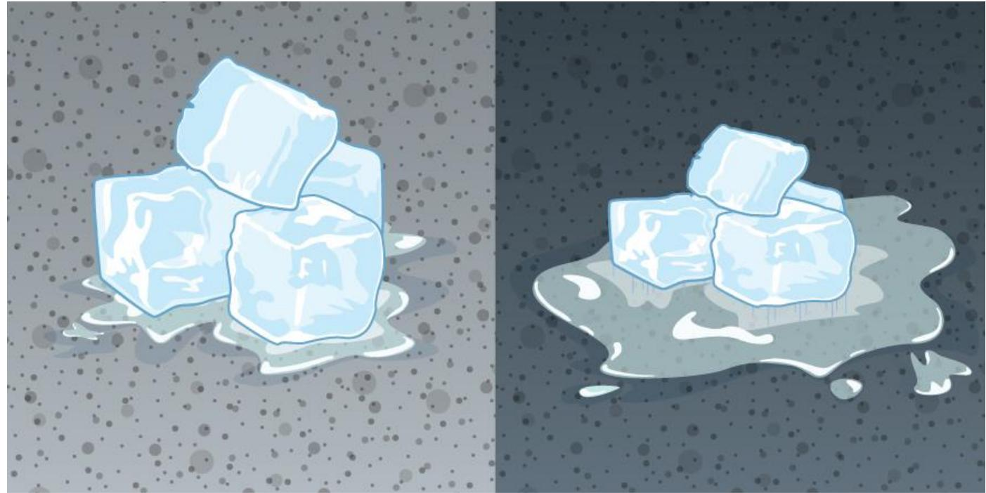
A darker object becomes hotter than a lighter-colored object when both are exposed to sunlight for the same amount of time and have the same thermal conductivity. This occurs because darker surfaces absorb more incident radiation, whereas lighter surfaces reflect a larger fraction of the incoming radiation.
