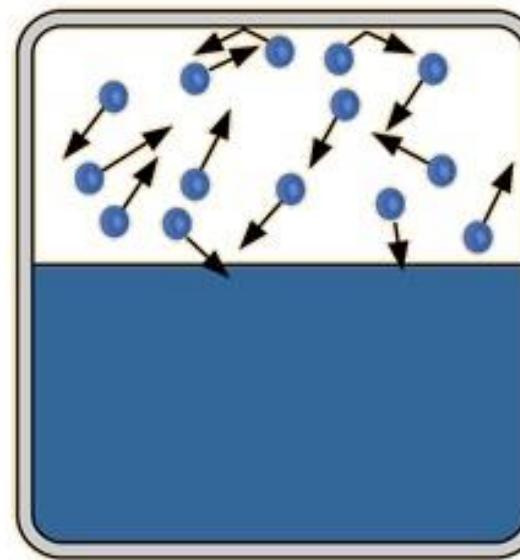
Evaporation which has reached equilibrium with the liquid surface is said to have reached saturation.
