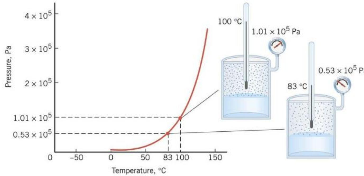
A point on the phase curve represents a condition where the liquid and vapor phases coexist in equilibrium.
